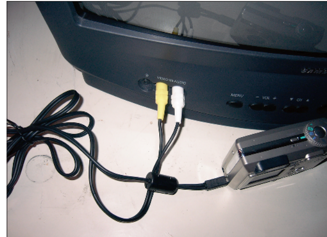
Figure 17-25: Hooking a camera to a TV
